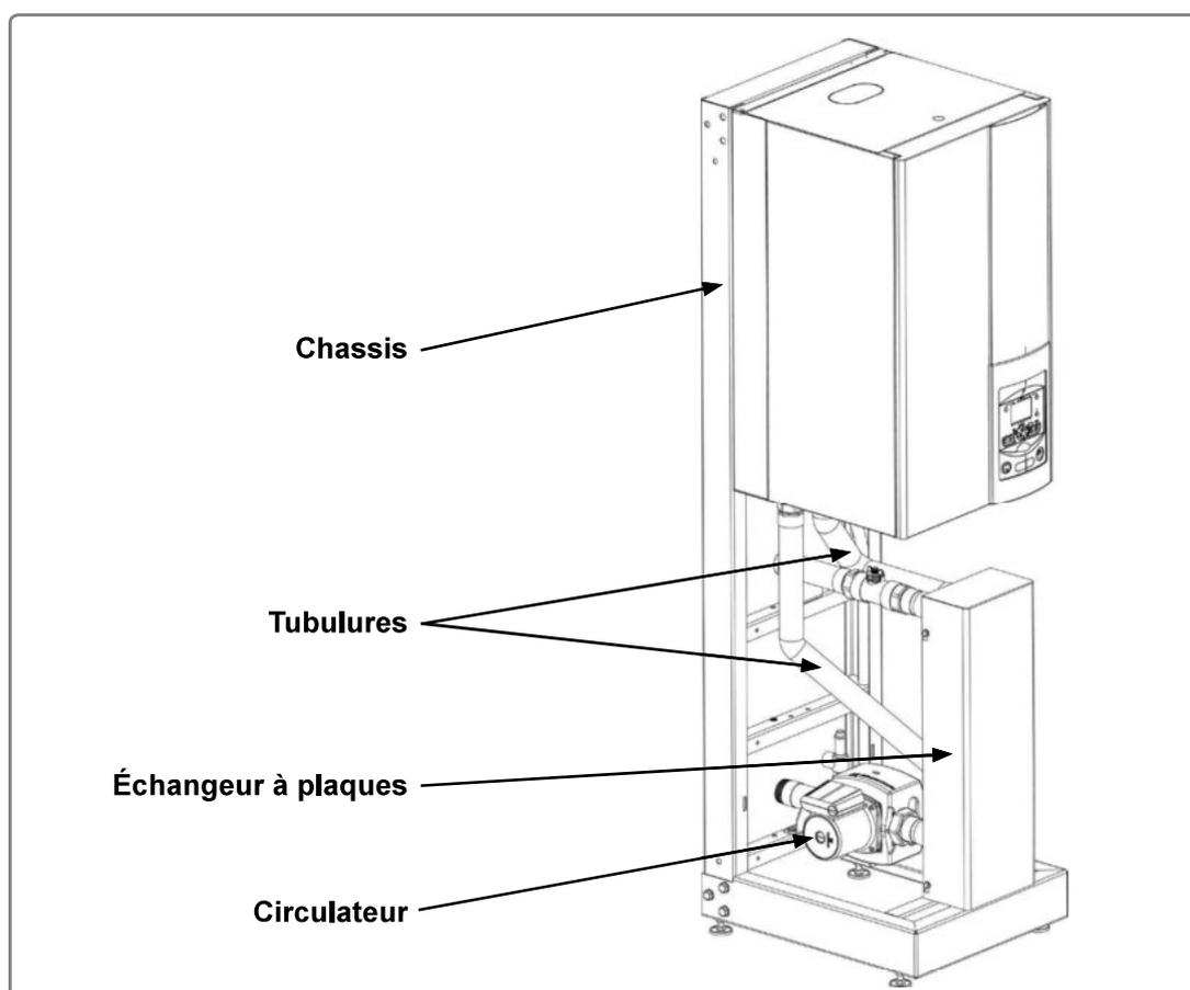
figure 8 - Module hydraulique
