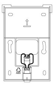
**Important:** The two wires of the data bus (A, B) may not be changed!
