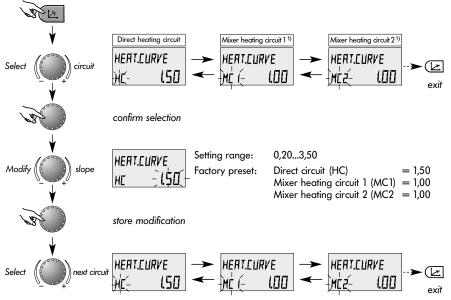
This button regulates the heating characteristics of each heating circuit in relation to outdoor temperature.
