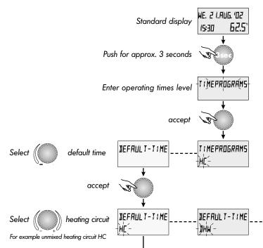
The standard programs do not get lost by overwriting with individual programs. Individual programs however are cancelled at a later call of the corresponding standard programs and have to be set up again. For this purpose individual switching-on and switching-off times should always be noted (see page 20/21).
