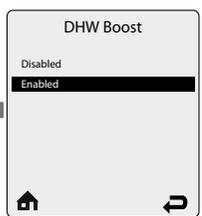
**DHW Boost**, when enabled, allows to increase the maximum DHW setpoint from 75°C to 85°C, provided that the DHW Setpoint menu is increased accordingly (see [page 16](#)).
