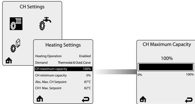
**CH Maximum Capacity** limits the maximum CH capacity. The appliance capacity can be defined by adjusting this value, 100% means Maximum CH output, 0% means minimum CH output. It is therefore possible to adjust the CH capacity to the installation needs.
