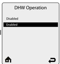
**DHW Operation** allows the domestic hot water function to be enabled and disabled. Touch the **UP** or **DOWN** soft keys to select Enabled or Disabled then touch the **OK** key to store the setting.
