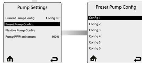
In the **Preset Pump Config.** (preferred selection) you can choose from a number of preset pump configurations. Only the configurations usable with a certain model/type of appliance will appear in the list. The configurations are detailed in "[System Diagrams and Set-up](#)". Each configuration is detailed through one or several hydraulic diagrams, a table indicating the electrical connections and a list of the parameters to be defined in ACVMax.
