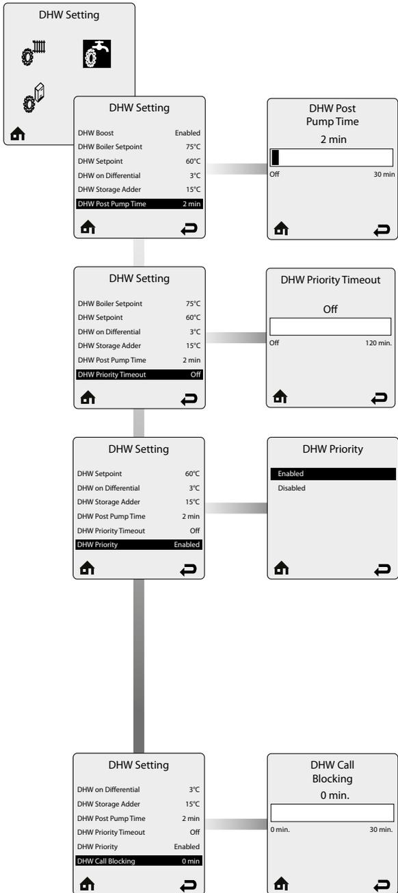
**DHW Post Pump Time** sets how long the domestic hot water circulator will continue to operate at the completion of a domestic hot water call. Any call during the DHW Post Pump Time will be ignored until the post pump has completed. The DHW Post Pump feature allows the heat remaining in the appliance at the completion of a call to be sent to the Indirect Water Heater, which will improve the overall efficiency of the system.
