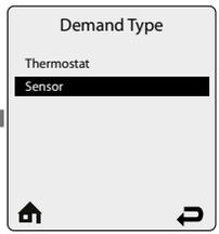
**Demand Type** allows to select the type of device that will generate a domestic hot water call. Touch the **UP** or **DOWN** soft keys to select the DHW Demand Type then touch the **OK** key to store the setting.
