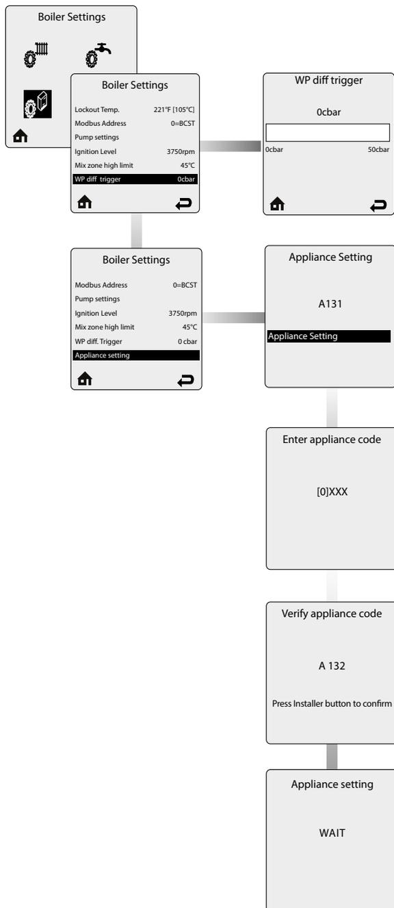
The **WP diff trigger** parameter is the required pressure change when the internal pump is starting. This function allows to detect the correct operation of the appliance internal pump.
