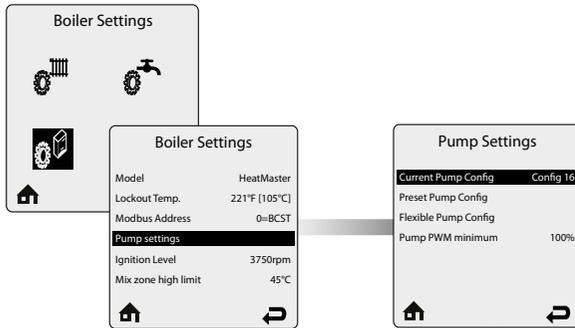
The **Pump Settings** menu allows to choose the right pump configuration to the chosen hydraulic configuration.
