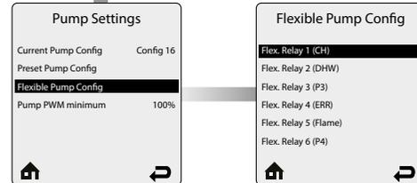
The **Flexible Pump Config.** menu allows to customize the connection of the pump(s) installed in the primary circuit in the chosen hydraulic configuration. Only select this option when the preset configurations do not offer you a solution. In this menu you have to choose, per relay, for which heat demand / function it will be activated. The relays are allocated as follows by default ( see picture below for physical location on the optional terminal blocks ) :
