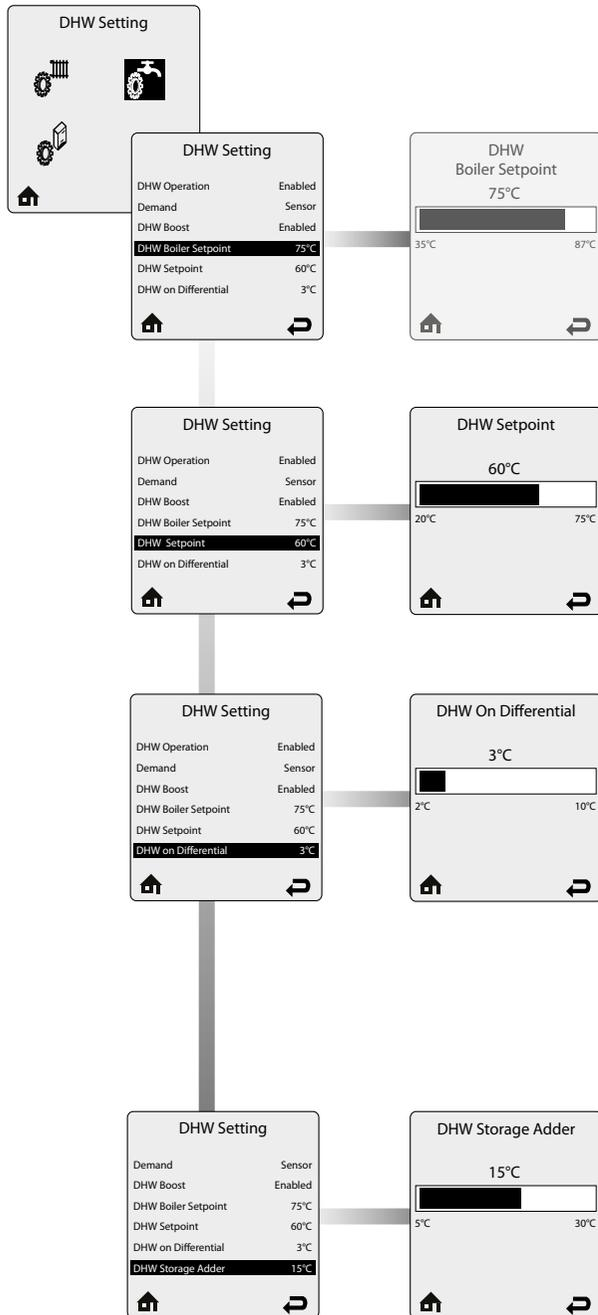
**DHW Boiler Setpoint** is the fixed appliance setpoint temperature during a domestic hot water call when the Thermostat option is chosen in Demand Type.
