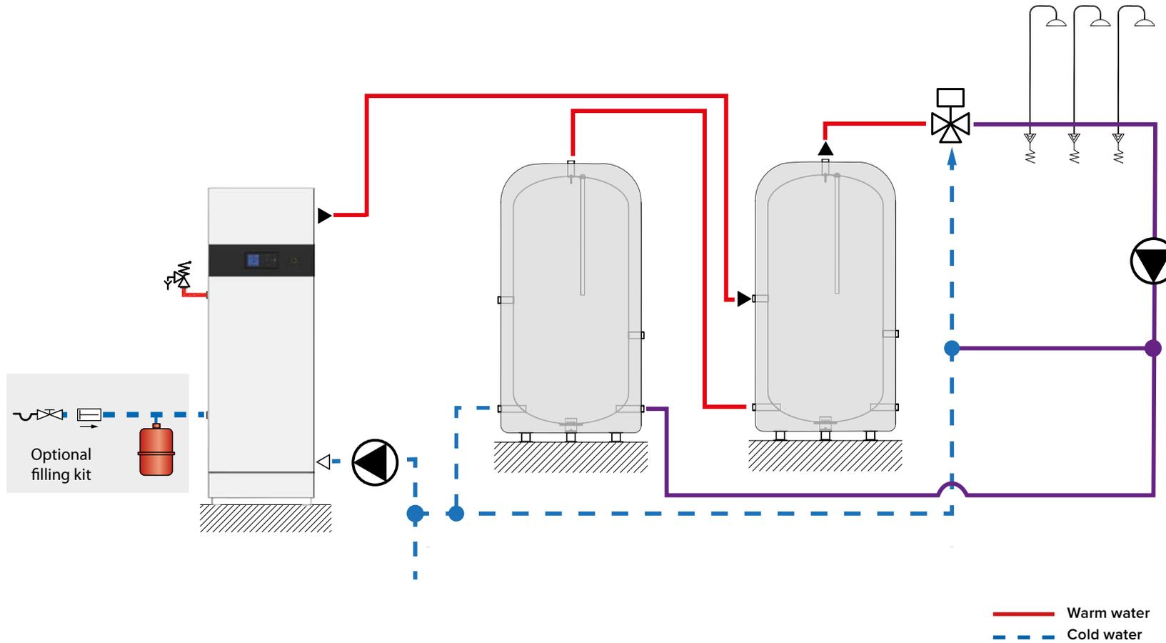
Two WaterMaster water heaters for the production of Domestic Hot Water, with two DHW buffer tanks and a recirculation circuit.
