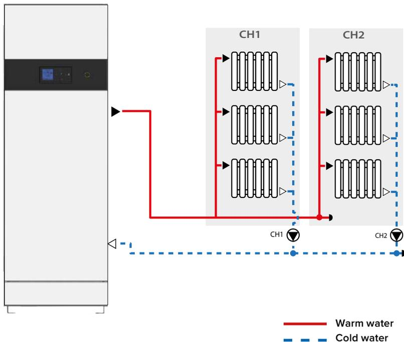
**i** Installing a three way valve in the heating supply will allow to control the temperature of the water supply to the heating system. Please contact your ACV representative for more information.
