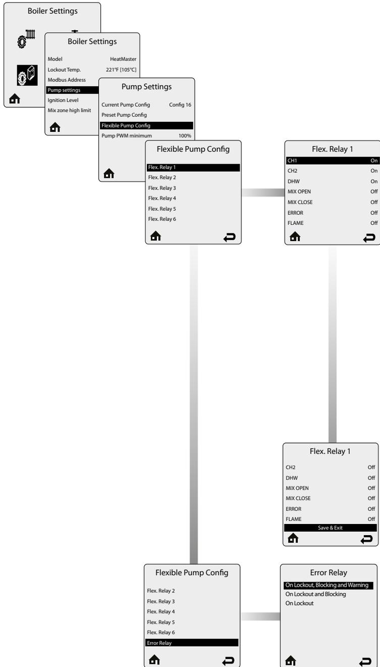
Each relay function has several options. Activation will happen when one of the following options has been chosen: **CH1, CH2, DHW, MIX OPEN, MIX CLOSE, ERROR, FLAME.**
