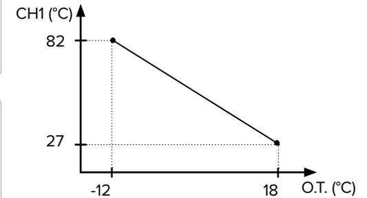
**Outdoor Curve Coldest Day** is the coldest outdoor design temperature of the heating system when an Outdoor Curve option is chosen in Demand Type. This setting is not applicable when a Setpoint option is chosen in Demand Type.
