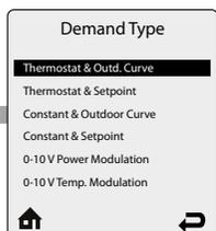
To navigate on the screen, use the **UP, DOWN, LEFT** and **RIGHT** keys
