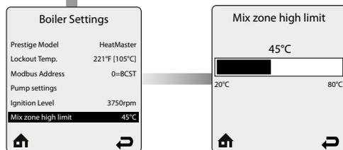
The **Mix zone high limit** setting allows to limit the maximum temperature in the mixed circuit. The function works like an Overheat Cut-off Activation of the limit and will cause the appliance to go in fault state (lockout). This setting allows to change the limit temperature for the mixed circuit. It is based on the CH1 setpoint.
