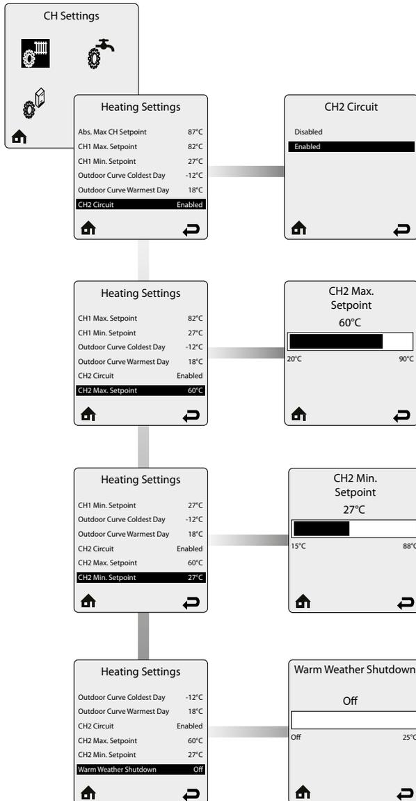
**CH2 Circuit** allows the CH2 heating call to be enabled and disabled.
