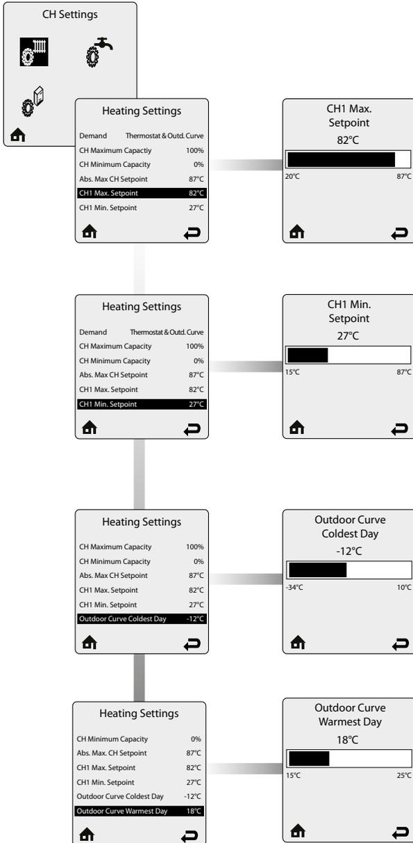
**CH1 Max. Setpoint** is the maximum setpoint for a CH1 heating call when an Outdoor Curve option is chosen in Demand Type. CH1 Maximum Setpoint is the fixed setpoint for a CH1 heating call when a Setpoint option is chosen in Demand Type.
