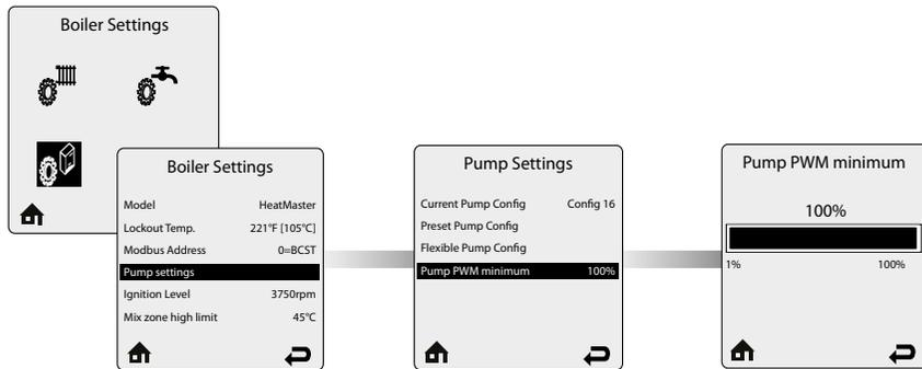
The **Pump PWM minimum** function allows to adjust the minimum pump setting if the flow in the appliance / system is insufficient at minimum appliance rate.
