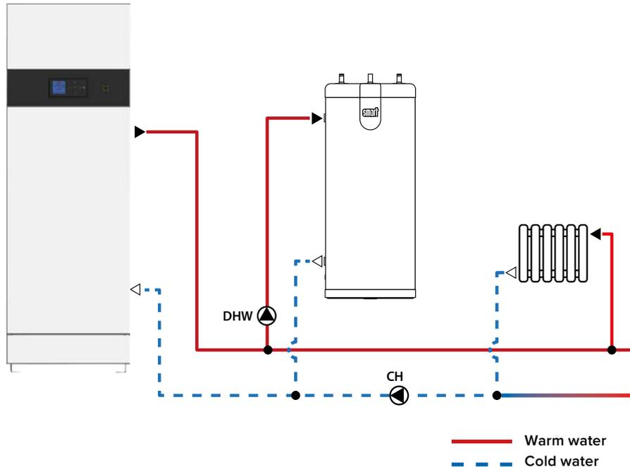
**i** Installing a three way valve in the heating supply will allow to control the temperature of the water supply to the heating system. Please contact your ACV representative for more information.
