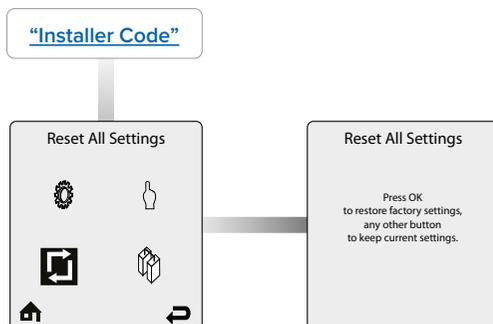
**Reset All Settings** allows the installer to reset all parameters back to the default values (Refer to [“Factory settings and reset values”](#) for the default settings).
