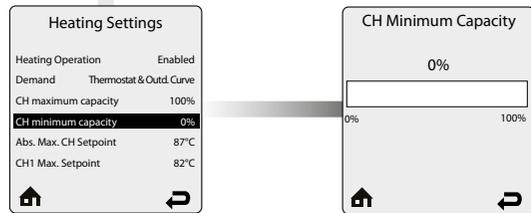
**CH Minimum Capacity** sets the lowest limit of the CH capacity. The appliance capacity can be defined by adjusting this value and the CH Maximum capacity. It is therefore possible to adjust the CH capacity to the installation needs.
