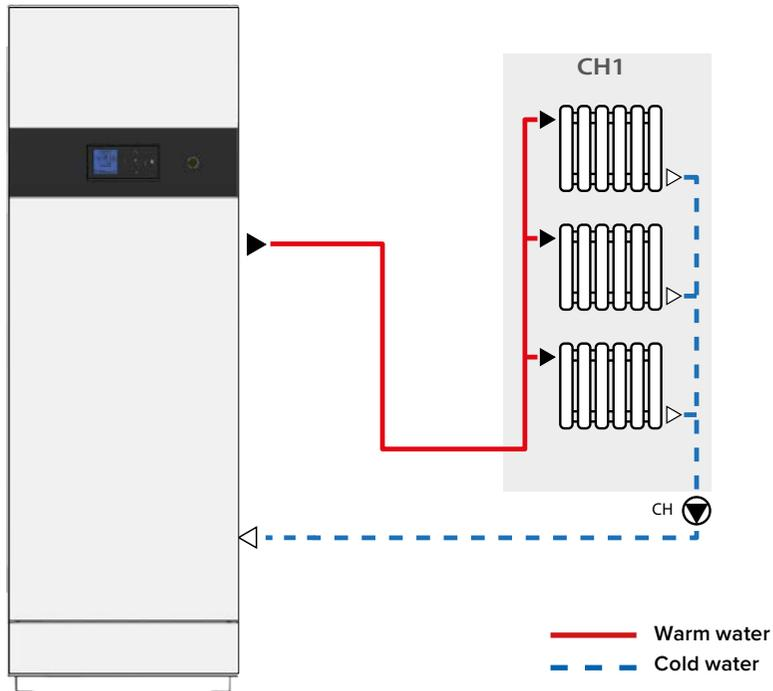
**i** Installing a three way valve in the heating supply will allow to control the temperature of the water supply to the heating system. Please contact your ACV representative for more information.
