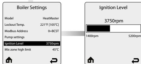
The **Ignition Level** parameter allows to change the fan start speed of the appliance.
