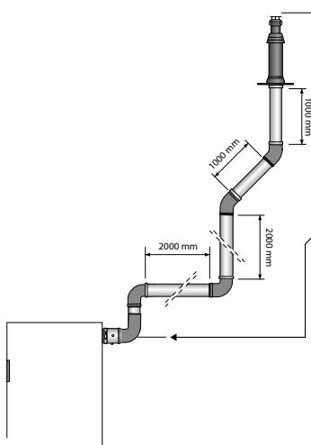
**Example of verification of the flue pipe length (L) in a concentric flue pipe system for HeatMaster 35 TC Evo (80/125):**
