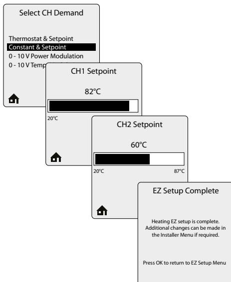
**Constant & Setpoint** - The HeatMaster will maintain setpoint without an external CH call from a thermostat or zone panel. The setpoint will be fixed for CH calls. After Constant & Setpoint is selected, the CH1 Setpoint screen appears.
