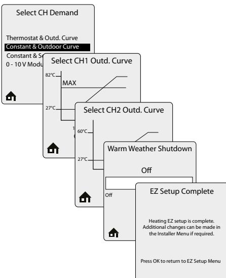
**Constant & Outdoor Curve** - This option is only displayed when the outdoor temperature sensor is connected. The HeatMaster will maintain the setpoint without an external call from a thermostat or zone panel. The setpoint will vary with the outdoor temperature for central heating calls.
