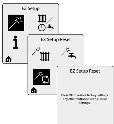
**EZ Setup Reset** allows to reset all EZ setup settings back to the original factory defaults.
