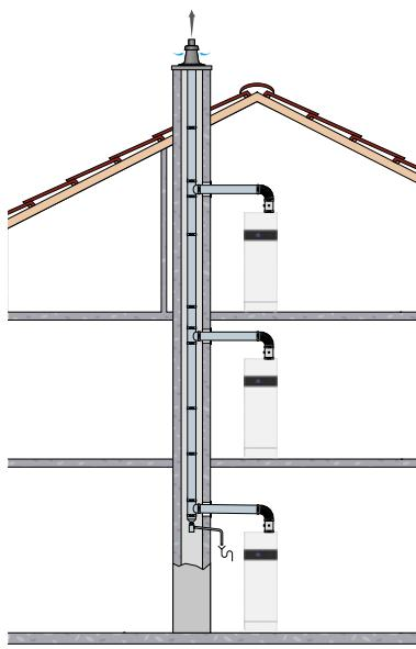
**HeatMaster 25 - 35 TC Evo cascade in a C43 chimney connection configuration**
