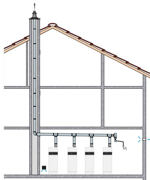
**HeatMaster TC Evo cascade in a B23 chimney connection configuration**
