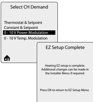
**0 - 10V Power Modulation** - This option allows the HeatMaster firing rate to be controlled by an external control system.
