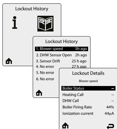
**Lockout History** records the last eight lockouts. Six lines are displayed on the Lockout History screen at one time. Each line contains a lockout description followed by how long ago the lockout occurred.
