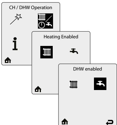
**CH/DHW Operation** provides a simple way to enable/disable either the CH or the DHW function of the HeatMaster.
