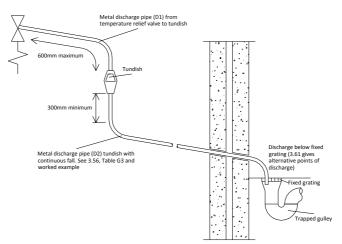
G3: Typical discharge pipe arrangement
