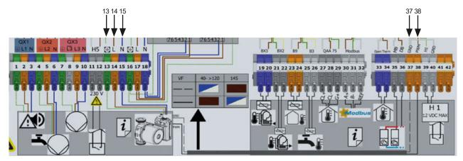
Figure 1 - Pump electrical connections
