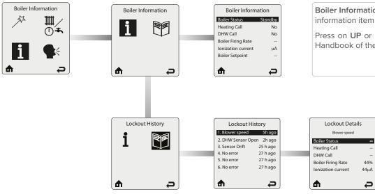
**Boiler Information** screen provides real time operating information of the Prestige. Each line contains an information item followed by its current value. Six lines are displayed on the screen at one time.
