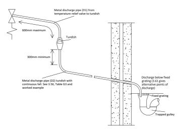
G3: Typical discharge pipe arrangement
