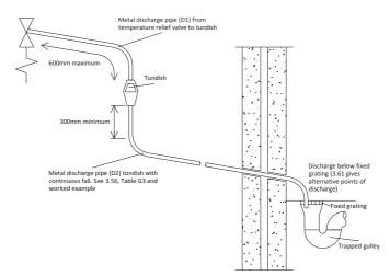
G3: Typical discharge pipe arrangement
